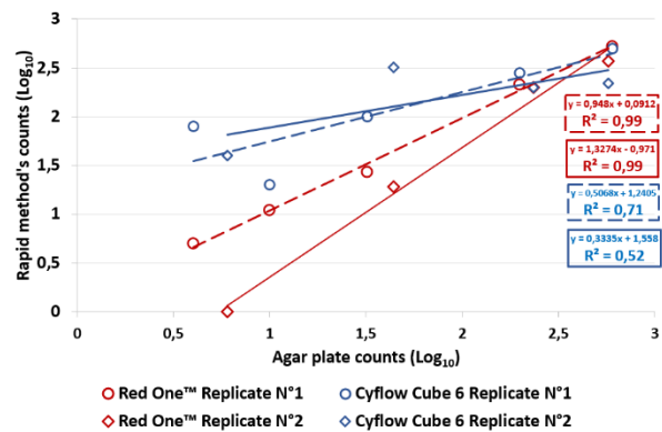
Figure 6: Correlation between Red One™; or CyFlow™ Cube 6 and agar plate counts for dilutions from 5 \times 10^0 to 5 \times 10^2 CFU/mL
